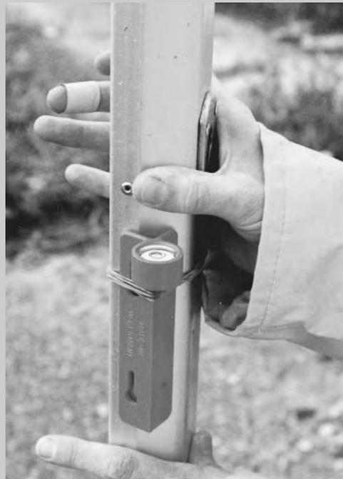
Figure 4.16 on page 111). Staffs for EDMs and total stations have a built-in air bubble so you can make sure they are level. Second, you will have to ensure that you have not rotated the face of the staff away from the telescope. Watch the direction in which the staff is facing and be prepared to adjust it if the surveyor can't read it clearly.
