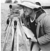
collimation is 61.4 metres. If you don't know the precise height above sea level of your datum then you will have to assign an arbitrary height to it (for instance, 100 metres. Don't make it zero or you'll end up with negative numbers). The sum of the first reading and the datum height is the value for the line of collimation (otherwise known as the **height of the instrument [HOI]**).
